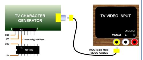
Only the first 3 pins are required for a basic connection. The complete setup is shown including the TV set, and these are the minimum connections required to start working with this unit. If a faster serial communication is required, selecting the appropriate combination of S1 and S2 will change the speed. This can be done at any time, just make sure that there is no data transmission while the change is executed.
